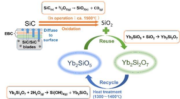
Fig. 2 Concept of recycle – reuse process for permanent self-crack healing ability
